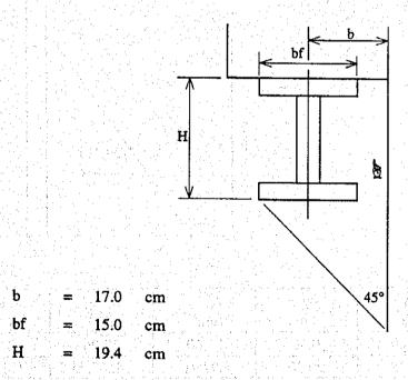
Shearing length of concrete: (L)
