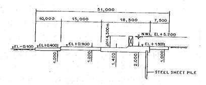
The length of sheet pile is calculated by using Lane's weighted creep theory as follows.
