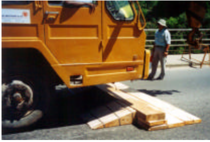
Photo 1 Vehicle drop test condition
