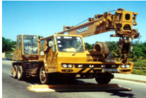
Photo 1 Vehicle drop test condition
