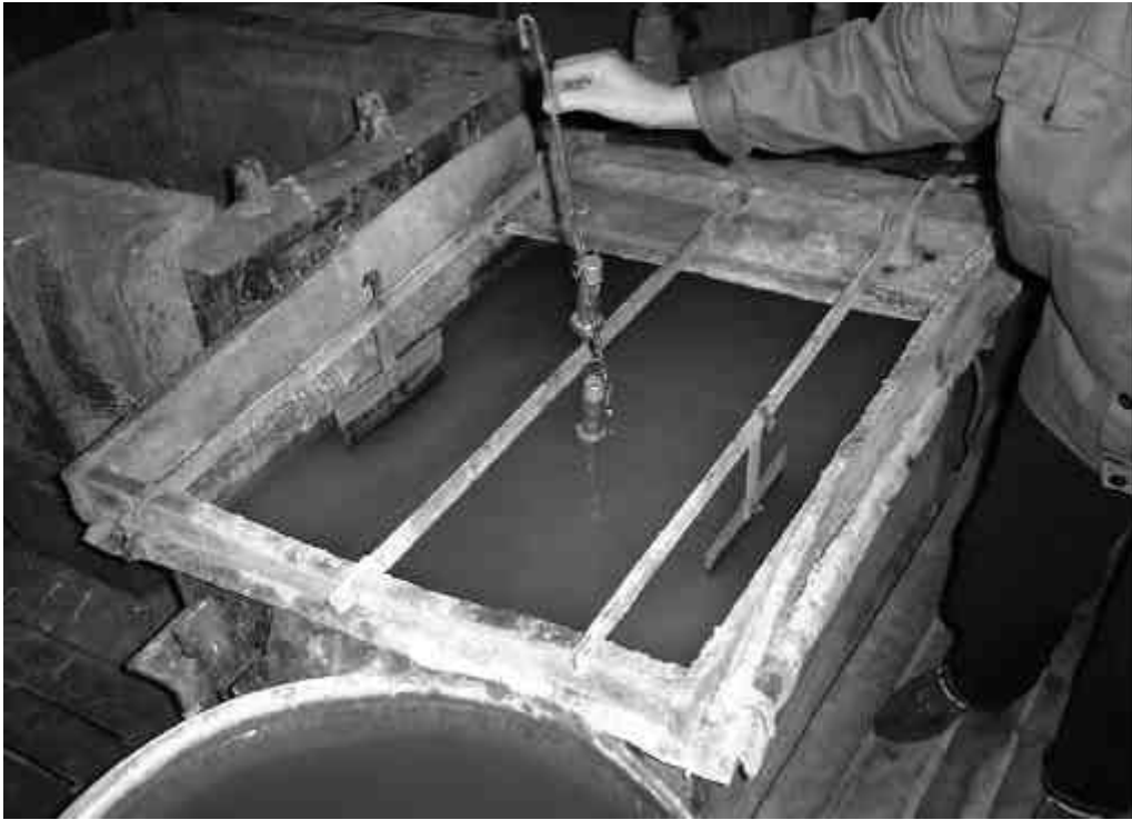
Plating Process / Zinc Plating Tank
