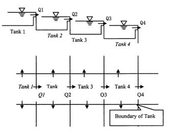
a tank to the next tank and the water level at the tank. The movement volume of discharge from a tank to the next tank within the calculation time interval ( $\Delta$  t) is controlled by the equation of motion, while the storage volume of the tank is by the equation of continuity. In this simulation, the following equations of motion and continuity are applied:
