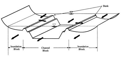
from the trunk drains and extensively inundates the flat low-lying hinterland. The flood flow will have various flow directions as illustrated in the conceptual figure above.
