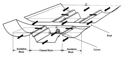
the road will have a flow direction toward downstream either over the road or through the culvert as illustrated above. In order to express the above flood channel flow and inundation conditions, the trunk drain and its surrounding flood inundation area are divided into the following blocks:
