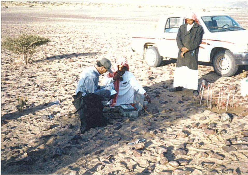
IP Survey: SCINTREX IPR-12 Time Domain IP/Resistivity Receiver
