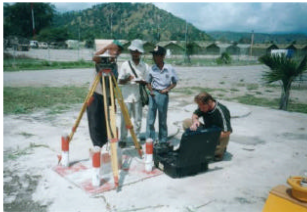
GPS observation in front of the control Tower at Comoro Airport (Reference point for horizontal coordinates)
