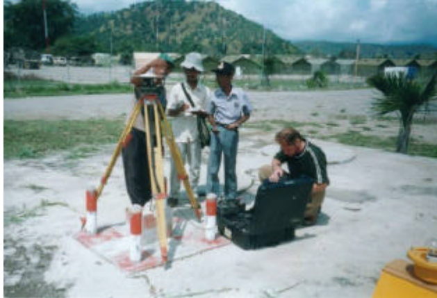
GPS observation in front of the control Tower at Comoro Airport (Reference point for horizontal coordinates)
