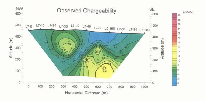
Figure 102 Observed IP cross-section (Line L7)
