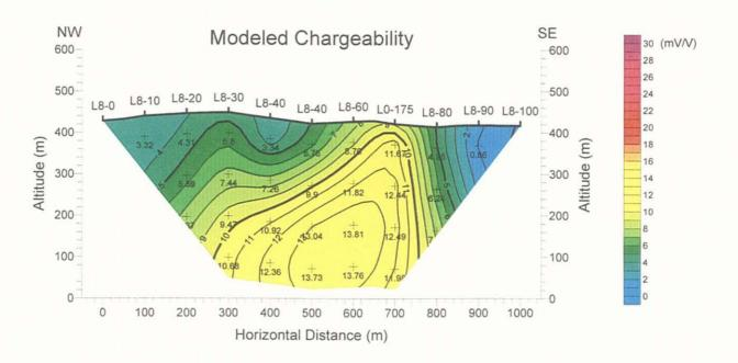
Figure 118 Modeled IP cross-section (Line L8)
