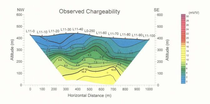
Figure 104 Ovserved IP cross-section (Line L11)
