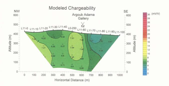
Figure 119 Modeled IP cross-section (Line L11)
