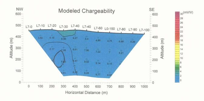
Figure 117 Modeled IP cross-section (Line L7)
