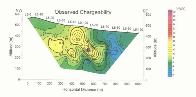
Figure 100 Observed IP cross-section (Line L5)
