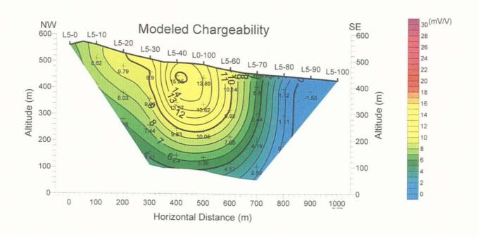
Figure 115 Modeled IP cross-section (Line L5)
