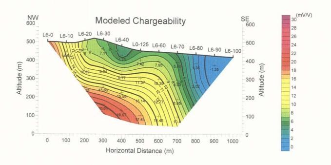
Figure 116 Modeled IP cross-section (Line L6)
