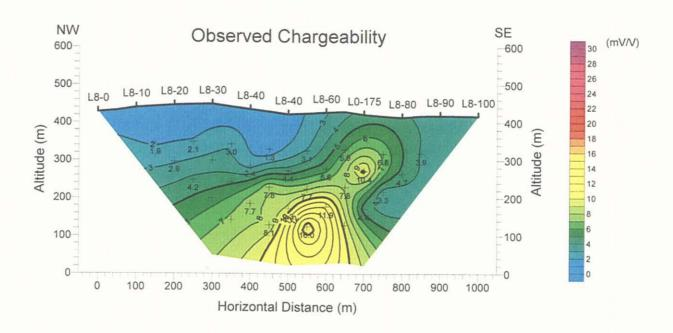
Figure 103 Observed IP cross-section (Line L8)
