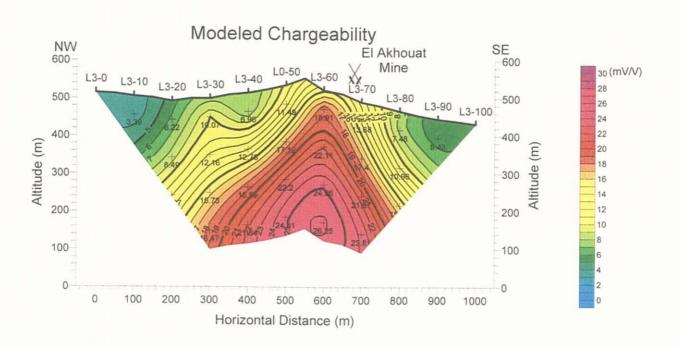
Figure 114 Modeled IP cross-section (Line L3)
