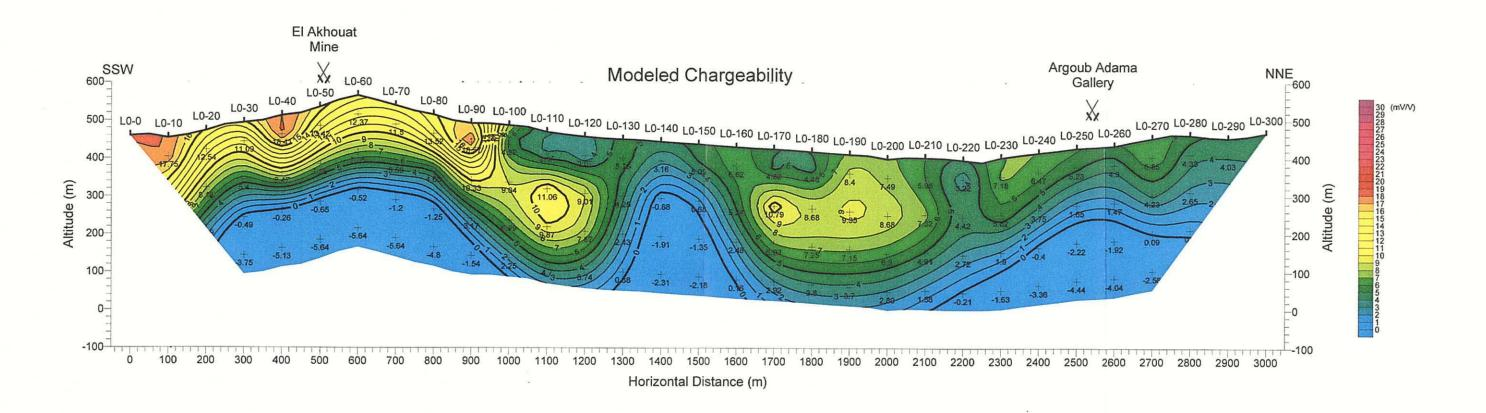
Figure 113 Modeled IP cross-section (Line L0)
