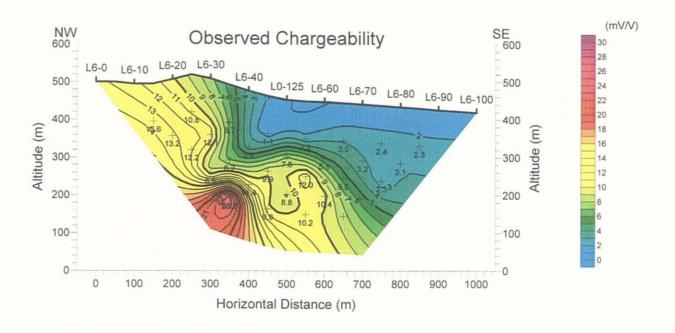
Figure 101 Observed IP cross-section (Line L6)
