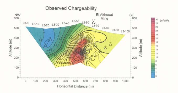
Figure 99 Observed IP cross-section (Line L3)
