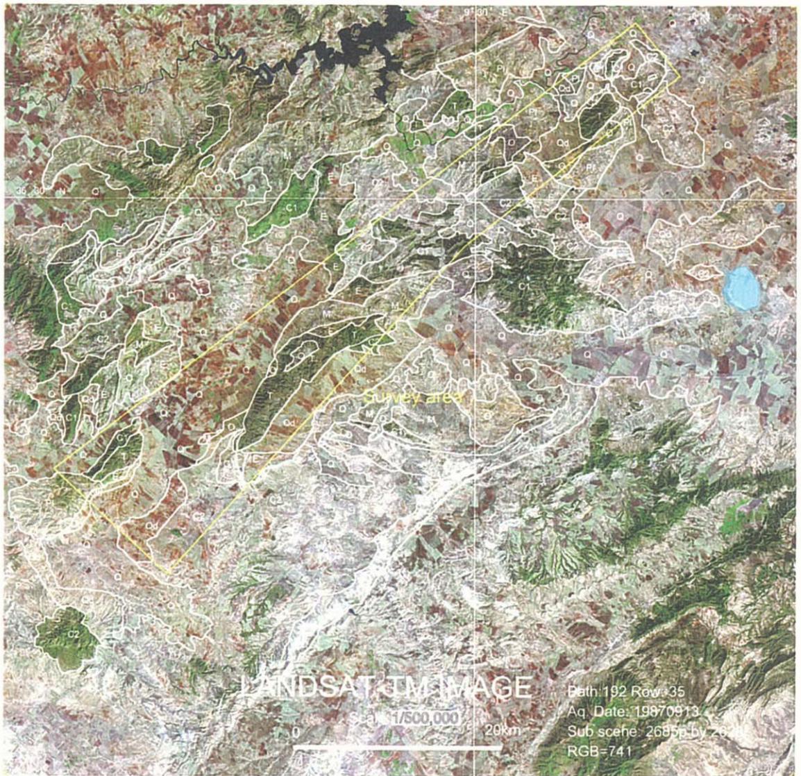
Figure 11 Interpretation map for rock phases of Landsat-TM image (RGB=7·4·1)
