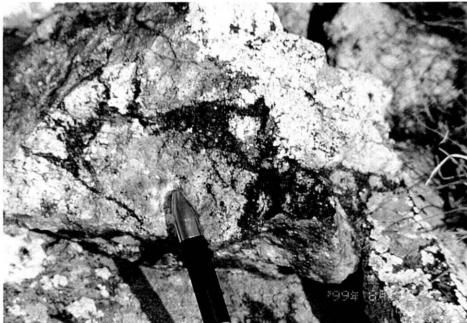
Plate 16 Fine grain tourmaline disseminates within matrix of brecciated syenogranite in No.42 Tourmaline prospect, Erdenet district.
