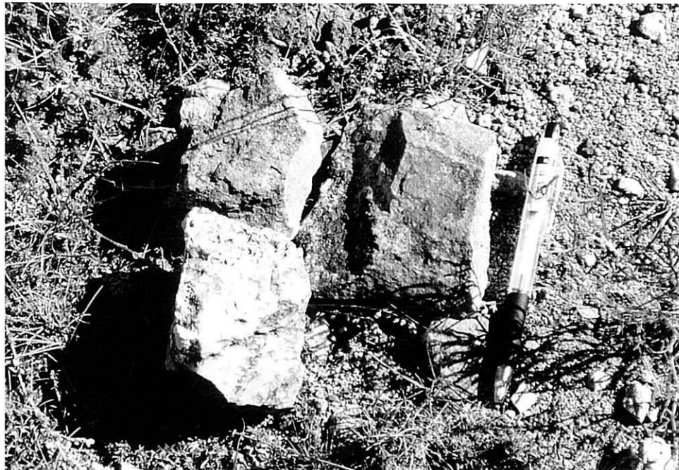
Plate 8 Potassic altered granite with Cu-oxide stain and quartz vein with chalcopyrite in No.32 Undrakh prospect, Bulgan West district.
