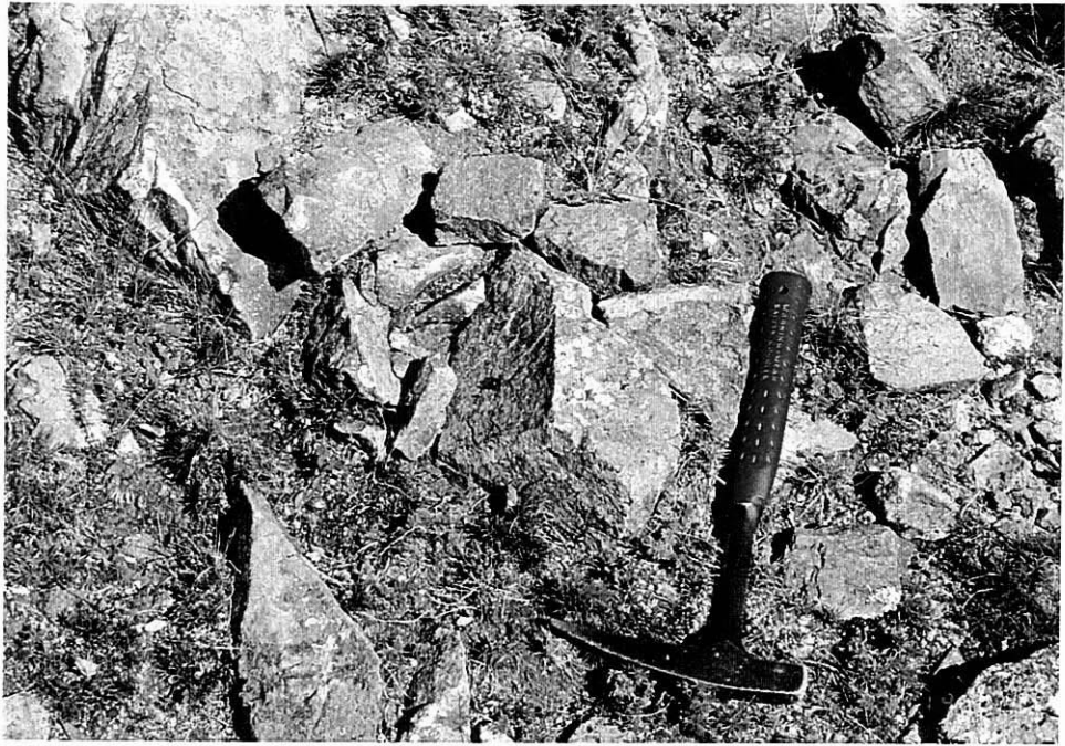
Plate 14 Weak silicified granite with Cu-oxide in No.41 Erdenet central deposit, Erdenet district.
