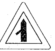
ທາງເຂົ້າທາງໂຕ້ຕອບ MERGE, LEFT WITH NON - PRIORITY ROAD W 33-2
