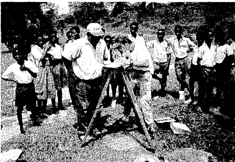
Eccentric observation using Planetable
