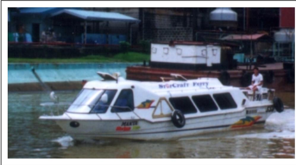
There are 19 such boats in operation. Unfortunately, many have been damaged by debris chipping or clogging of propellers. Almost three-fourths of the boats are out of commission at any one time. Larger catamaran-style boats originally designed for Laguna de Bay are now plying the river.
