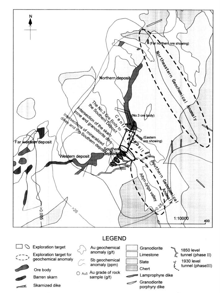
Fig. III-1-1 Exploration Targets in Altyn-Jylga Ore Field
