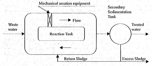
Treatment of wastewater in a low-load condition (BOD-SS load is 0.03 ~ 0.05 kgBOD /kgSS,day), oxidation ditch treatment process is characterized by long solids retention time and by nitrifying reaction increasing, it is also possible to remove nitrogen by providing an anoxic zone.
