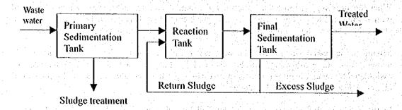
The characteristics of conventional activated sludge process are shown below:
