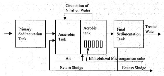
Biological wastewater treatment systems use the effect of microorganism activity. Because of this, to shorten a treatment time or to achieve higher treated water quality, it is necessary to maintain usable number of microorganisms in the reaction tanks by increasing the microorganisms concentration and the retention time of microorganisms in the reaction tanks.
