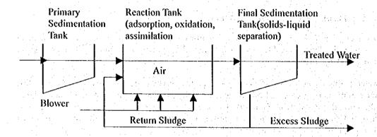
Two processes that are most widely used for the biological wastewater treatment are:
