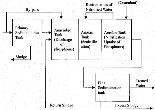
For the average water quality of urban wastewater, it is expected for primary sedimentation tank effluent, that total nitrogen removal efficiency to be  $60 \sim 70\%$ , and total phosphorus removal efficiency to be  $70 \sim 80\%$ .
