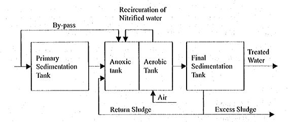
For average water quality of urban wastewater, removal efficiency of total nitrogen as annual average is expected to be  $60 \sim 70\%$  for primary sedimentation tank effluent, and also BOD and SS removal efficiency exceeds the conventional activated sludge process. Characteristics of recirculation nitrification-denitrification process are shown below:
