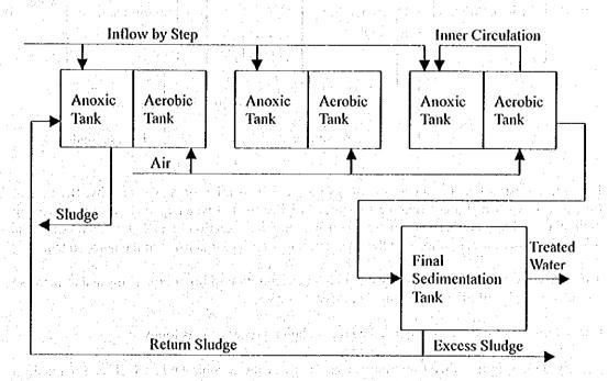
To add more steps to this process, air volume is increased because it is applied to denitrification reaction after the nitrification reaction, it is not necessary so many internal recirculation of mixed liquor. So it is not necessary to provide a circulation pumps, and also it is not necessary electric power for pumps.
