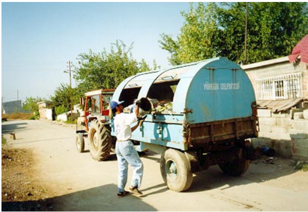
Municipal solid waste collection in Yuregir, where about 75 percent of collection vehicles are tractor trailers
