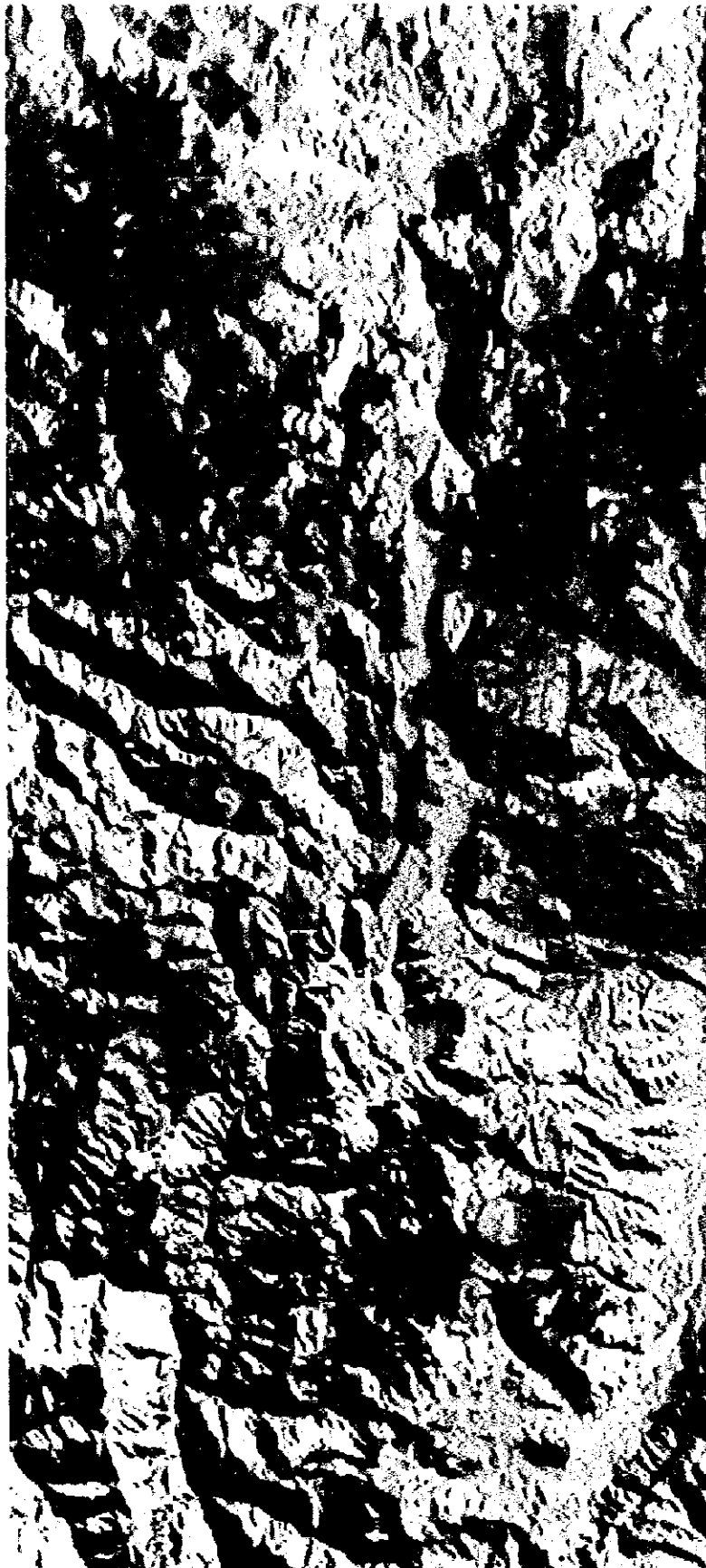
Figure II-1-19 Landsat TM false color composite of the Valle del Cura area, from a regional mosaic image in JICA/MMAJ/JMEC (1998). BGR:1+5.
