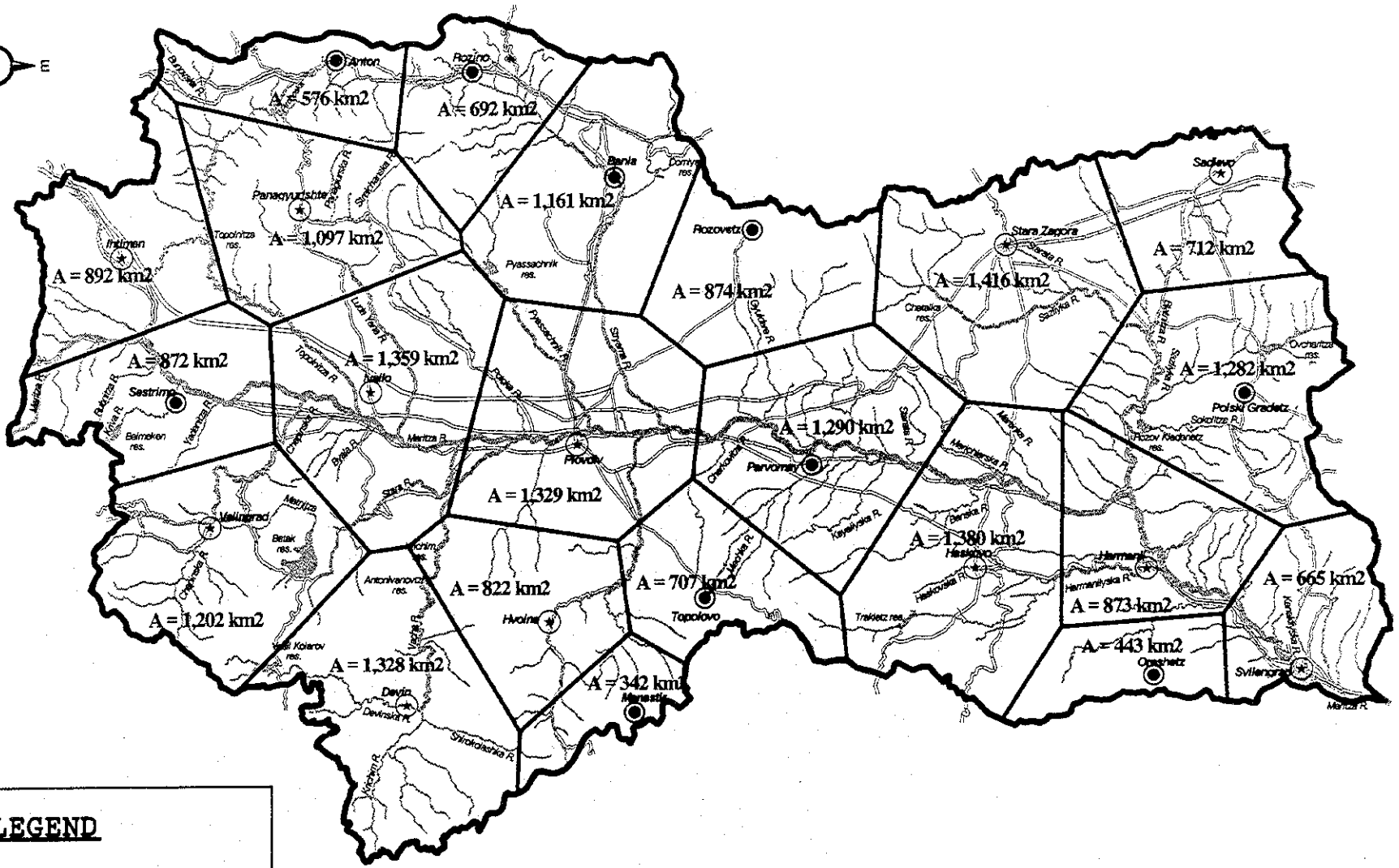
FIG.D.4.7 THIESSEN POLYGONS ASSOCIATED WITH THE REPRESENTATIVE STATIONS
