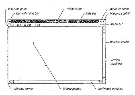
The *Control-menu* box located in the upper-left corner of the window is the most useful menu when the use of a keyboard is preferred. The Control-menu commands can resize, move, maximize, minimize and close windows, and switch to Task List.
