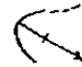
Direction of gentle dip and rim. Arrow should be extended to foot of slope.
