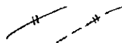
Hard bed of steep altitude, when direction of dip cannot be observed or may be to both directions. Frequent on hogbacks.
