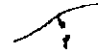
Downthrown side of fault direction of fault plane, dip and facet (D).
