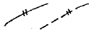
Hard bed of steep attitude, when direction of dip cannot be observed or may be to both directions. Frequent on hogbacks.
