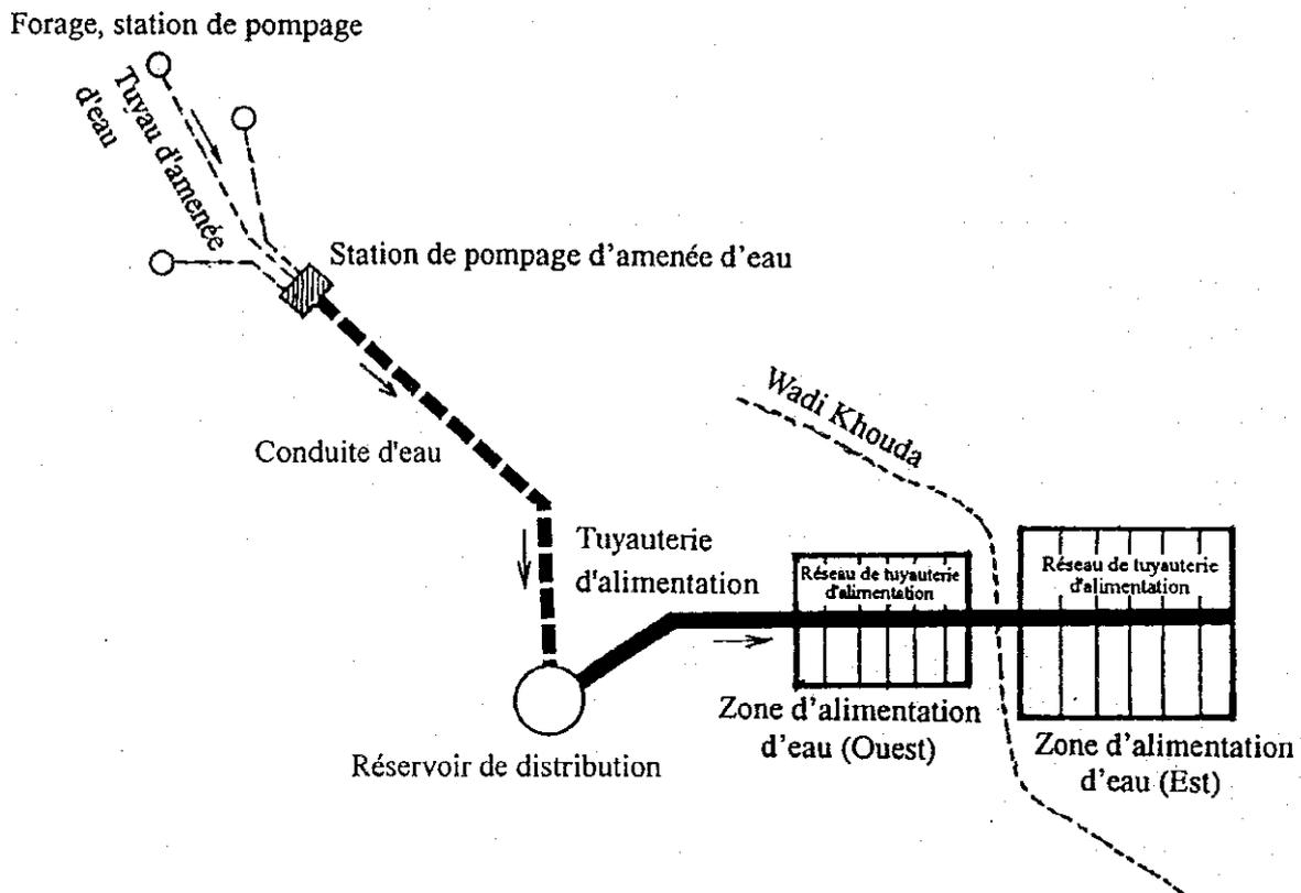
Fig. 5-1 Conceptual figure of water supply system
