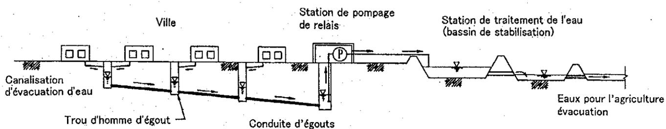
Fig. 6-1 Concept of sewage system servicing
