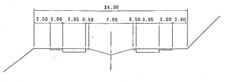
Fig. 6.4.6 Cross Section of New Road for 20 Mill. Ton/Year
