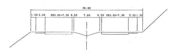
Fig. 6.4.3 Cross Section of Winding Road for 10 Mil. Ton/Year (4 Lanes)
