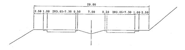
Fig. 6.4.7 Cross Section of New Road for 30 Mill. Ton/Year
