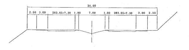
Fig. 6.4.8 Cross Section of New Road for 40 Mill. Ton/Year
