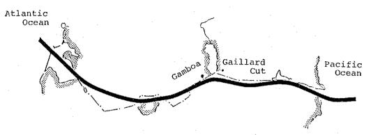
The figure show the Sea Level Canal alignment for Route-14S Entering from the Pacific Coast side, the Sea Level Canal route passes hilly areas through the continental divide, parallel to the existing canal zone through the Culebra Cut, then joins the existing canal near Gamboa.
