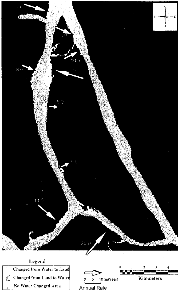
Fig. 6.14 Planform change of the Vam Nao Pass between 1972.12 to 1993.02
