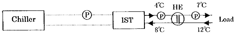
(b) Ice Discharge Operation
