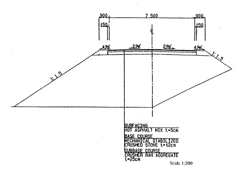
Figure 7.2 Typical Cross Section of Approach Road on the Embankment
