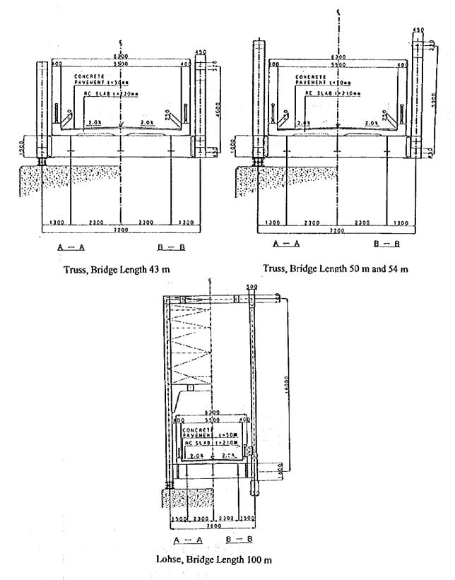
Figure 7.3 Bridge Cross Sections
