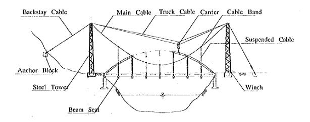
Fig.8.2 Cable Erection Method
