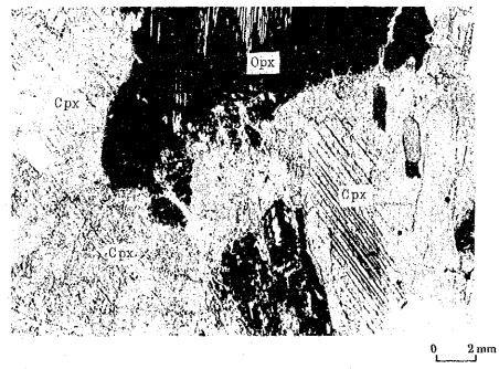
Gabbro (Sample No. SOR-22) Locality : 12 Km N of Brookes Point Main Mineral : Plagioclase, Clinopyroxene Accessory Mineral : Serpentine, Magnetite, Prehnite
