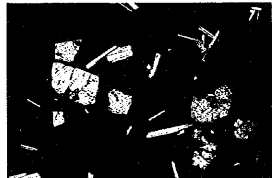
C : 97SMC04CB07-T1 Olivine basalt (porphyritic, glassy)
