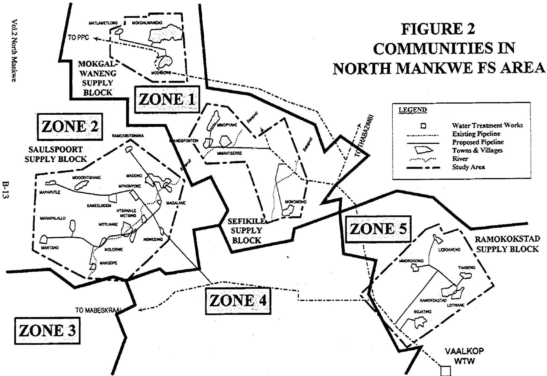
The details of the proposed infrastructure such as the need for booster pumping stations and their location, pipeline routes and the exact location of service reservoirs has yet to be determined however in general terms the communities will be supplied as follows.
