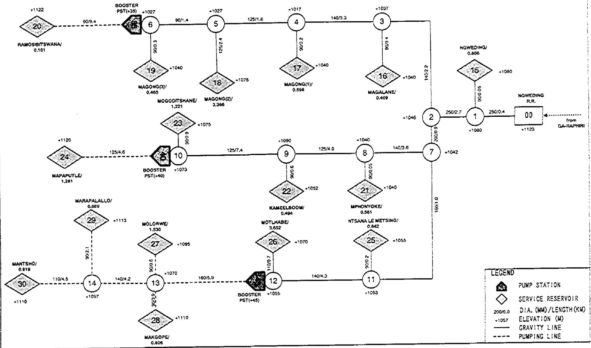
**FIGURE A.2-5 FLOW DIAGRAM IN SEFIKILE SUPPLY BLOCK**
