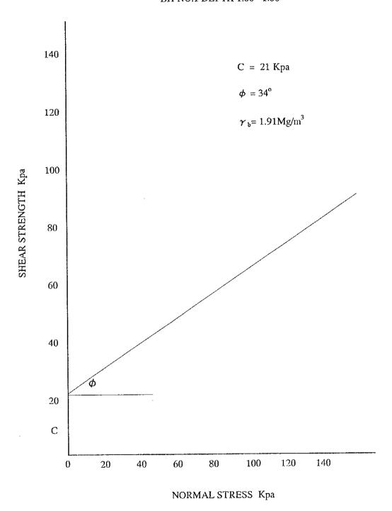
Result of Shear Strength Test (2) HOIMA ROAD (2) BH NO. 1 DEPTH:3.00 - 3.45m
