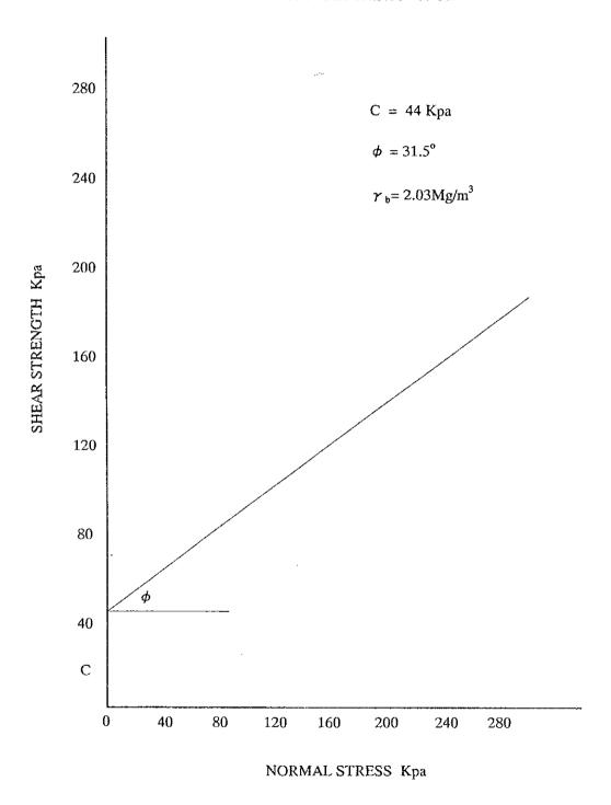
Result of Shear Strength Test (3) NATETE ROAD (1) BH NO.2 DEPTH:1.50 - 1.95m
