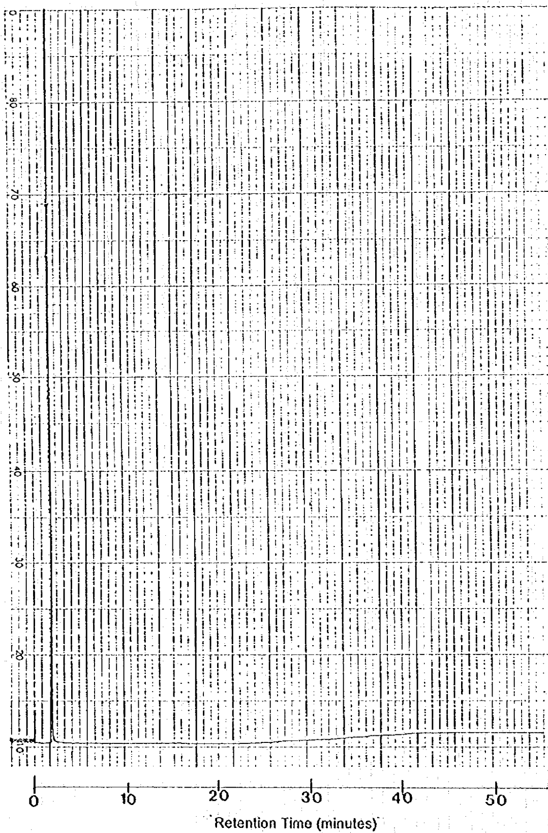
FIGURE (6): GC-ECD chromatogram of syringe solvent blank (hexane, hplc-grade).
