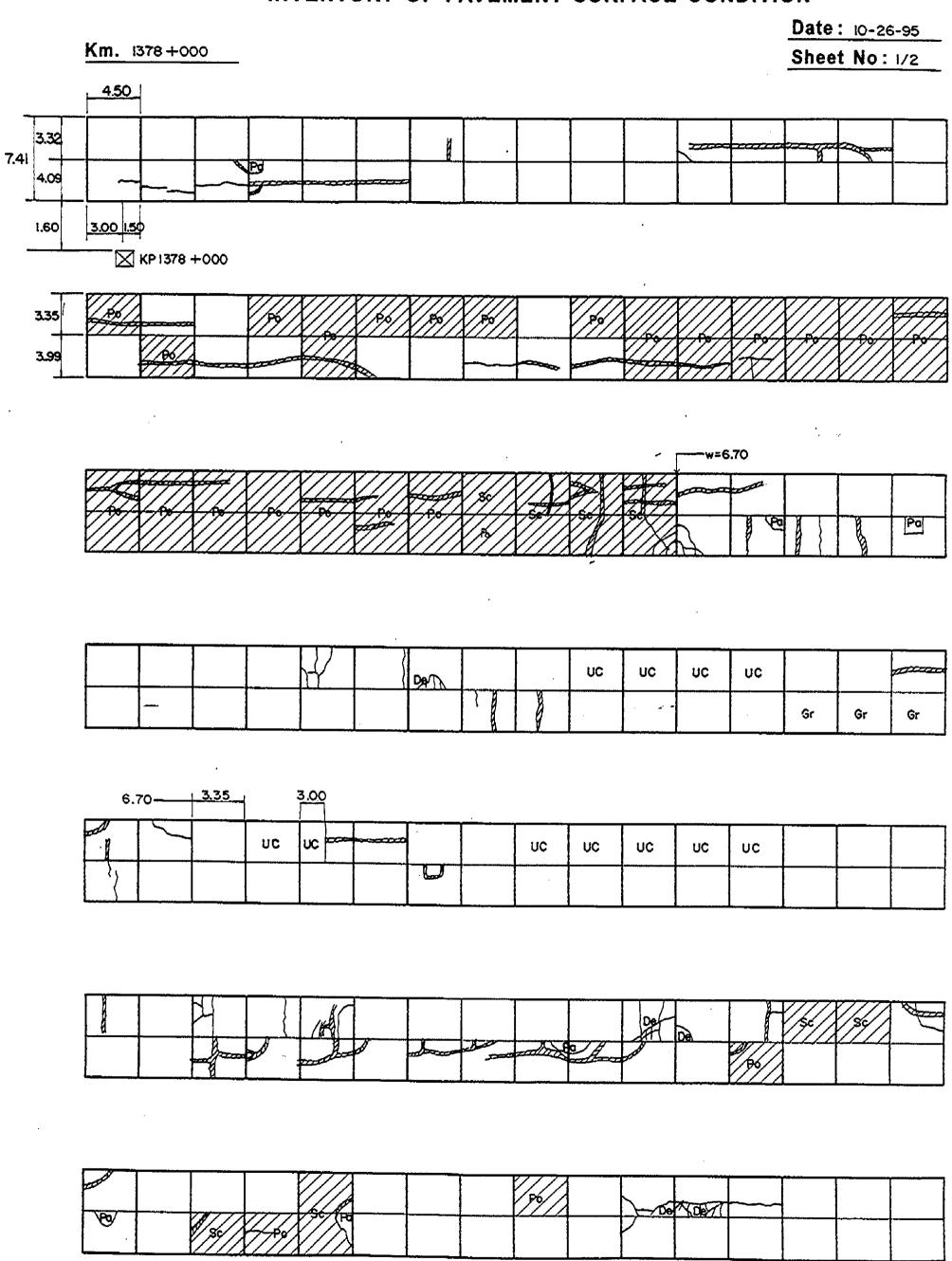
INVENTORY OF PAVEMENT SURFACE CONDITION Date: 10-26-95 Km. 1378+000 Sheet No: 2/2 UC UC UC ŲC UC UC UC 2.70 Under construction slope & embankment side Ģr Under const'n. slope 8 emb. side -Ģr G Gr De Gr Gr Gr 4.50 00 UÇ UC
