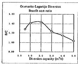
As illustrated above, both B-C and B/C are the maximum with the diversion capacity of 2 m<sup>3</sup>/s. The diversion capacity has been accordingly determined at 2 m<sup>3</sup>/s considering the higher value of B-C and B/C. The construction cost is estimated at
