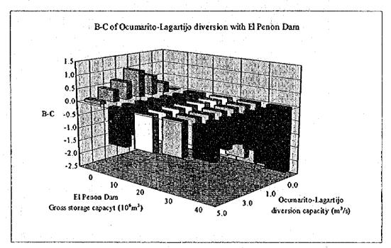
The following table shows the Annual Net Present Value (B-C), Benefit-Cost Ratio (B/C) and unit cost per cubic meters of water. The case with El Peñón Dam is the case with the effective capacity of  $30 \times 10^6 \text{m}^3$ , the best case among those with El Peñón Dam (for detail, see Table 4.3-4).
