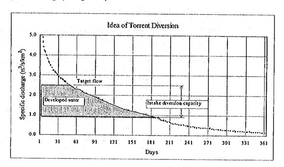
The water volume taken at the intake by target flow is as follows:
