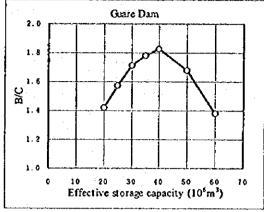
As illustrated above, both B-C and B/C are the maximum with the gross storage capacity of  $40 \times 10^6 \text{m}^3$ . The gross storage capacity has been accordingly determined at  $40 \text{ m}^3$ /s considering the higher value of B-C and B/C.
