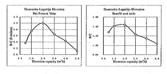
As illustrated above, both B-C and B/C are the maximum with the diversion capacity of  $2 \text{ m}^3$ /s. The diversion capacity is accordingly determined at  $2 \text{ m}^3$ /s considering the higher value of B-C and B/C. The construction cost is estimated at US\$19.44 million.
