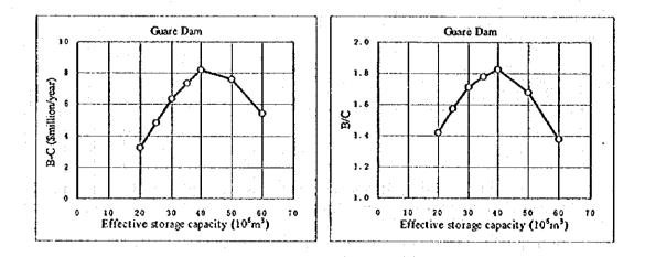
As illustrated above, both B-C and B/C are the maximum with the gross storage capacity of  $40 \times 10^6 \text{m}^3$ . The gross storage capacity has been accordingly determined at  $40 \text{ m}^3$ /s considering the higher value of B-C and B/C.
