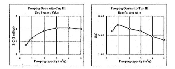
The Annual Net Present Value is the highest value with the pumping capacity of 4 m<sup>3</sup>/s while the benefit-cost ratio takes the highest value with a pumping capacity of 1 m<sup>3</sup>/s. The values of B/C are high in all cases at more than 3. The values of B-C for the pumping capacity of 3, 4 and 5 are almost the same. Accordingly, the pumping capacity of 5 m<sup>3</sup>/s is recommendable.
