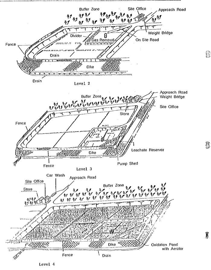
Figure 8-3: Illustration of Prospective Sanitary Landfill Development and Operation Levels 2, 3 and 4
