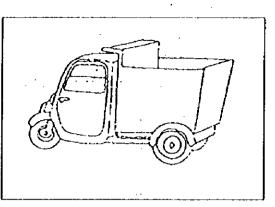
vehicles. Its relatively high speed gives this system an operating radius of about  $10 \text{ km}^4$ . However, tricycles do not operate well on rough, unpaved roads such as those in marginal areas or those which typically lead to disposal sites.
