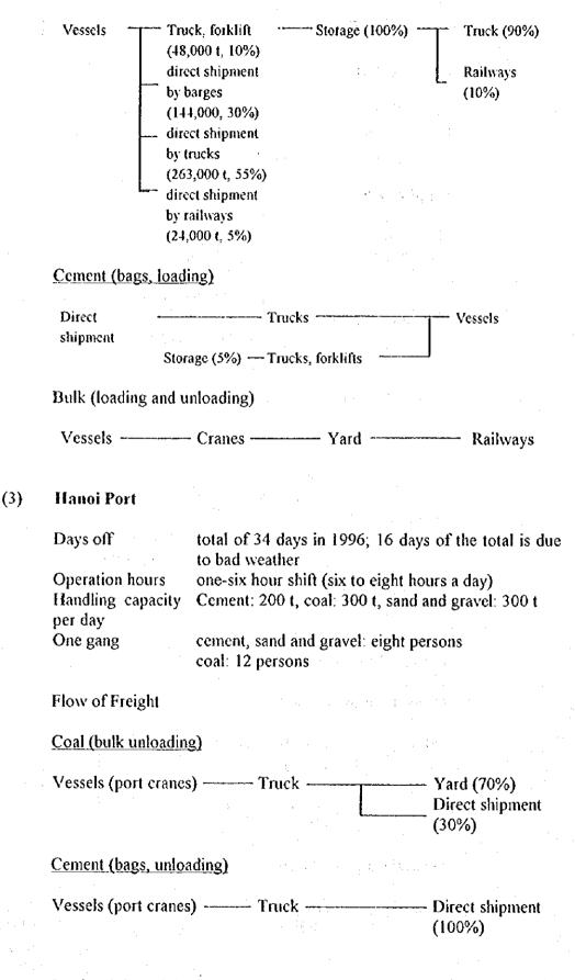
Sand and Gravel (bulk unloading)
