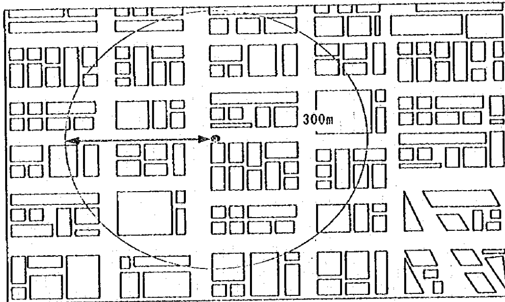
Figure 4.2 CS Coverage in Urban Area (CS is installed high)
