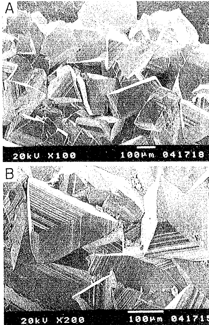
Fig. 11. SEM micrographs of chalcopyrite synthesized hydrothermally at 350°C, 300 kgf (H003). A, B: Tetrahedral crystals of chalcopyrite showing striation.
