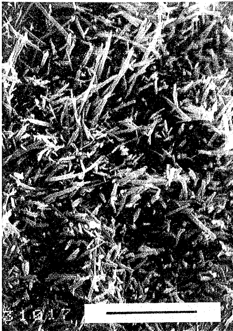
Fig. 8. SEM photomicrograph of tubular halloysite in kaolin ore. A bar of the scale is 5 microns long. Specimen No. 90062905. (The photomicrograph was taken by M. Aoki).
