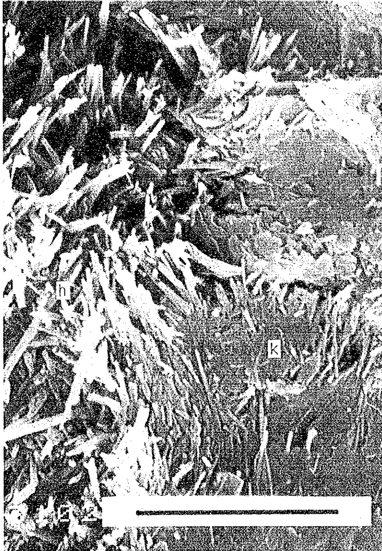
Fig. 10. SEM photomicrograph of tubular halloysite surrounding aggregate of platy kaolinite. h: halloysite, k: kaolinite. Bar scale 5 microns. Specimen No. 90062905. (The photomicrograph was taken by M. Aoki).
