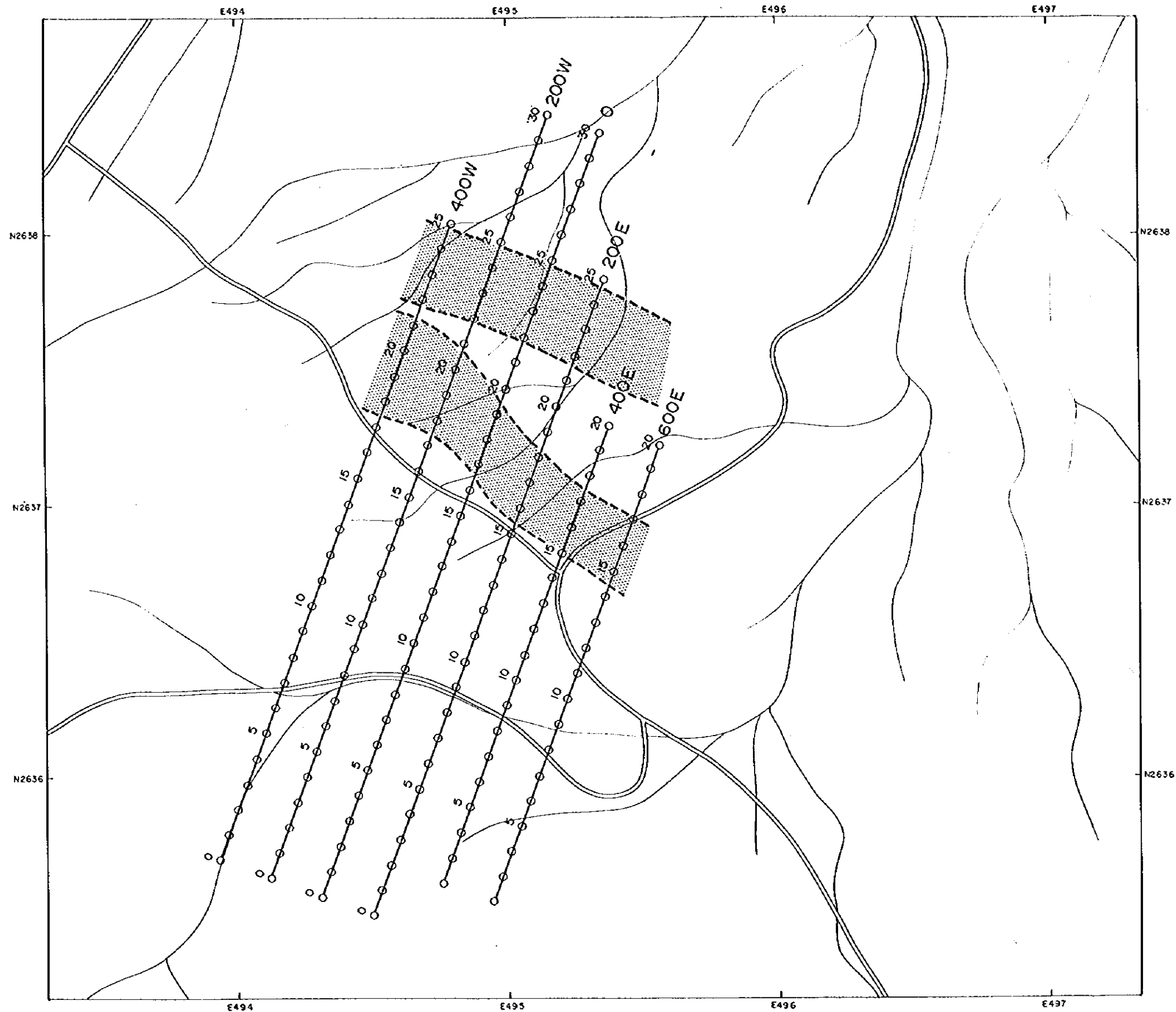
Fig. II-4-22 IP line locations in Ghuzayn West area
