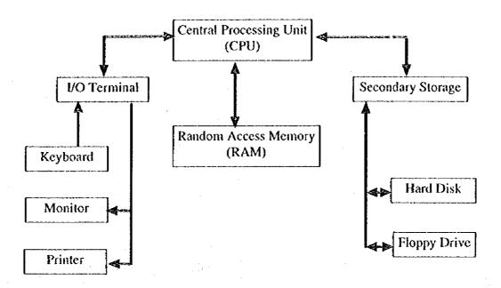
The diagram below presents the basic hardware component of a microcomputer system.
