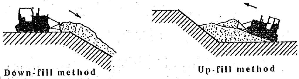
Fig. 5-2 Method of Bedding and Compaction
