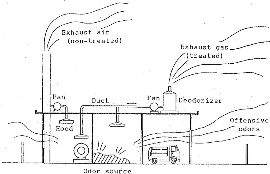
Figure 5-2 Schematics of Arrangement of Deodorization Facility
