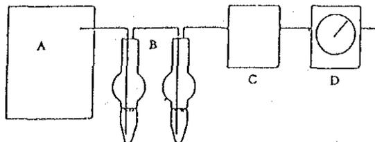
A: Sampling bag containing gas      B: Absorption bag
