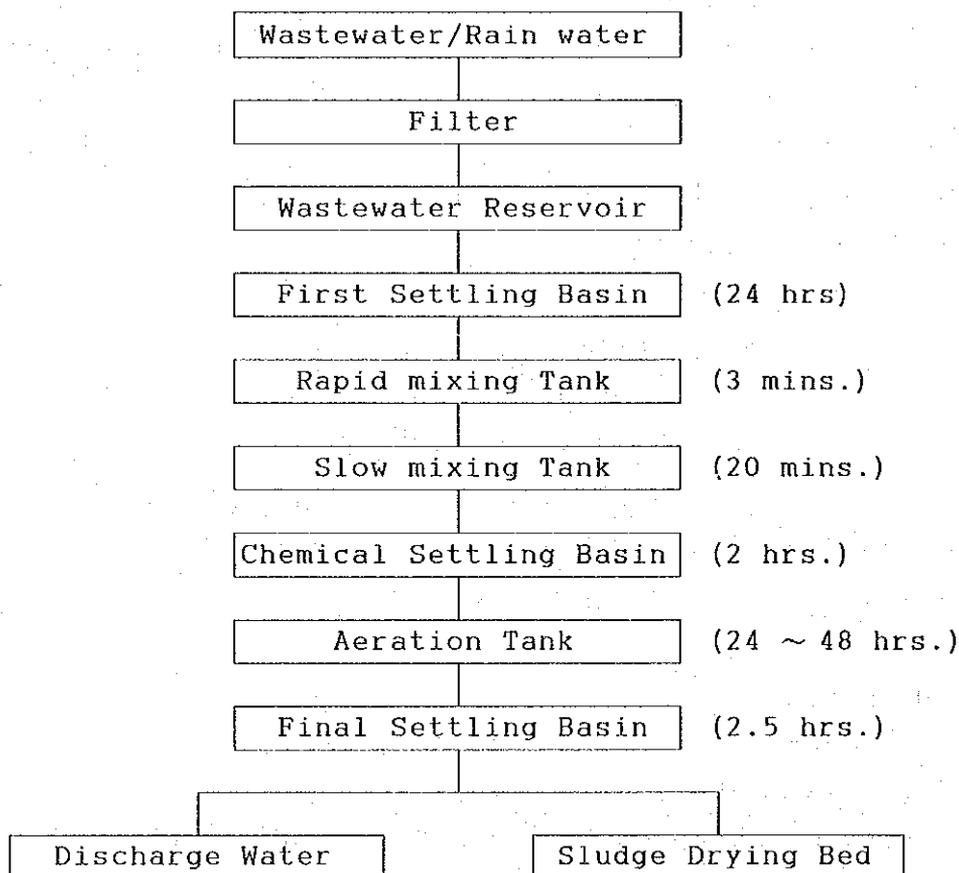
Figure 4-41 Treatment Process of Central Tanning Wastewater Treatment plant
