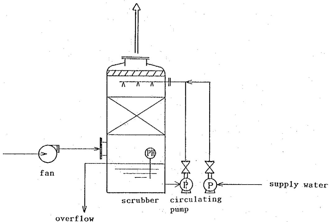
Figure 5-6 Schematic of Chemical Scrubbing
