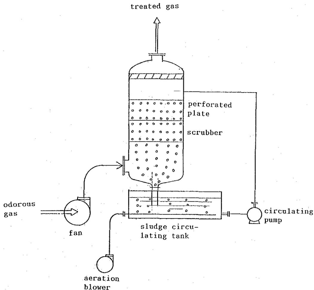
Figure 5-7 Schematic of Sludge Deodorization
