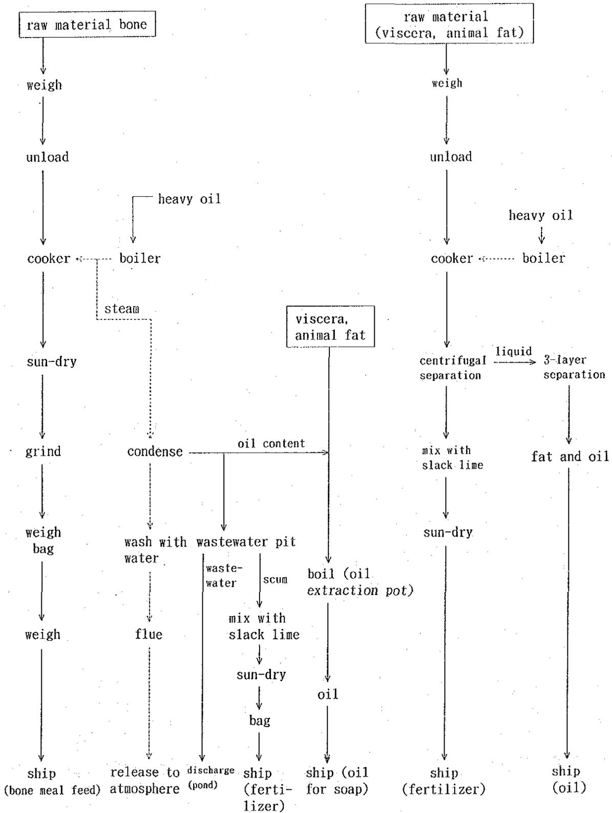
Figure 4-18 Production Process (Bone Meal Plant C)
