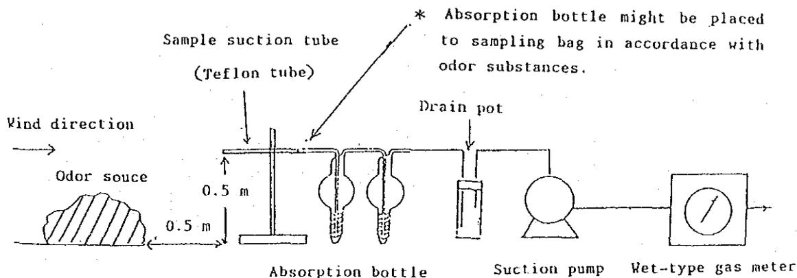
In case of gas sampling of odor source which was heaped up on the ground level, a sample suction tube was fixed on a holding stand leeward at a height and a distance of 0.5 m, and the sample gas was sucked through absorption bottle.
