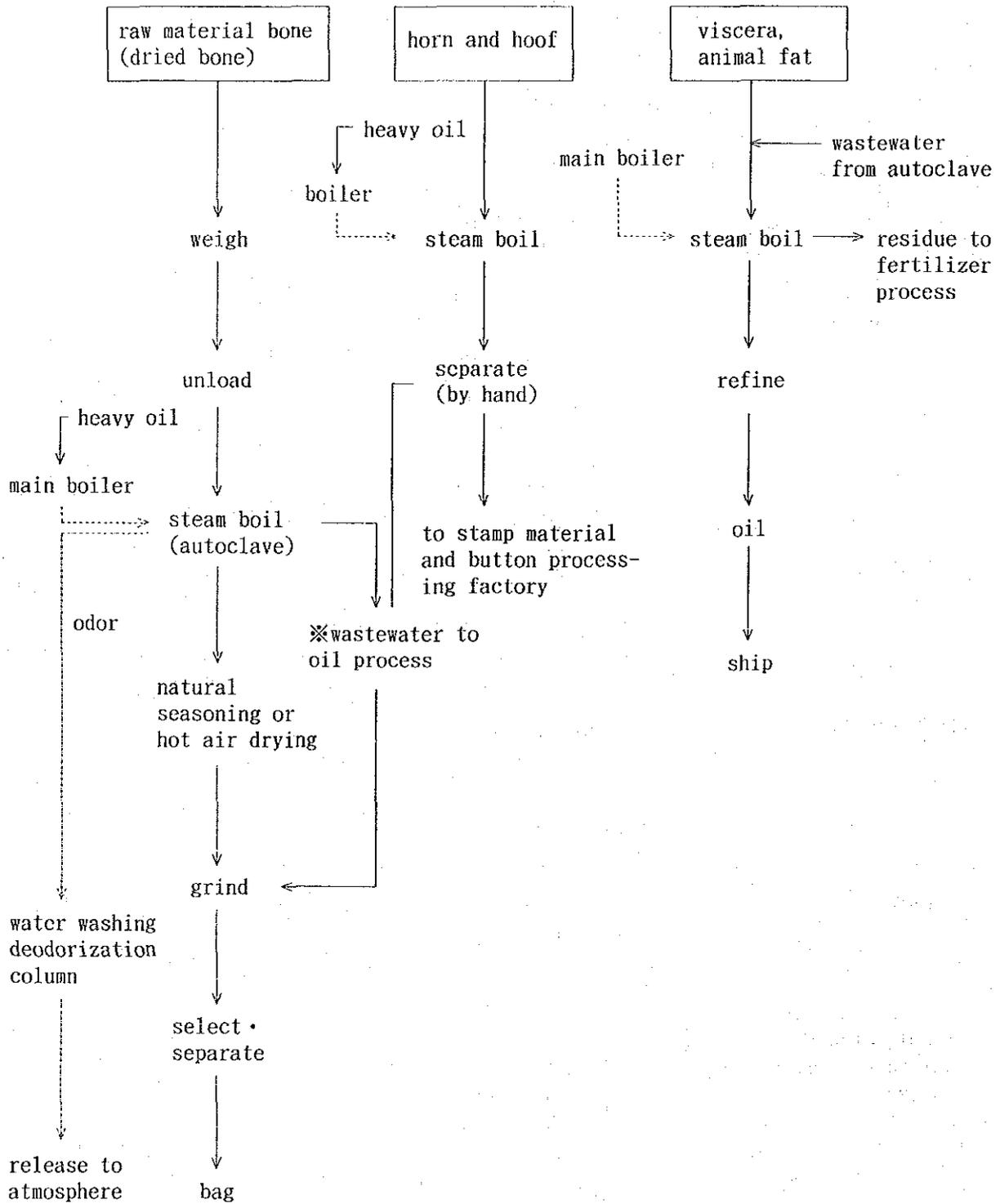
Figure 4-22 (2) Production Process (Bone Meal Plant D)
