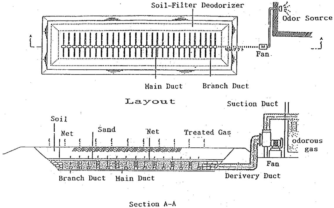
Figure 5-9 Schematic of Soil-Filter Deodorization
