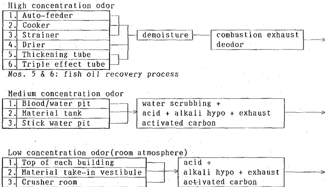
Figure 5-13 Deodorization Flow in Fish Meal Plant
