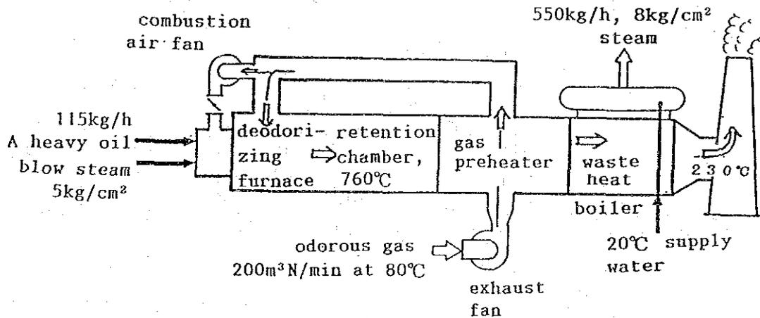
Figure 5-10 Schematic of Thermal Combustion
