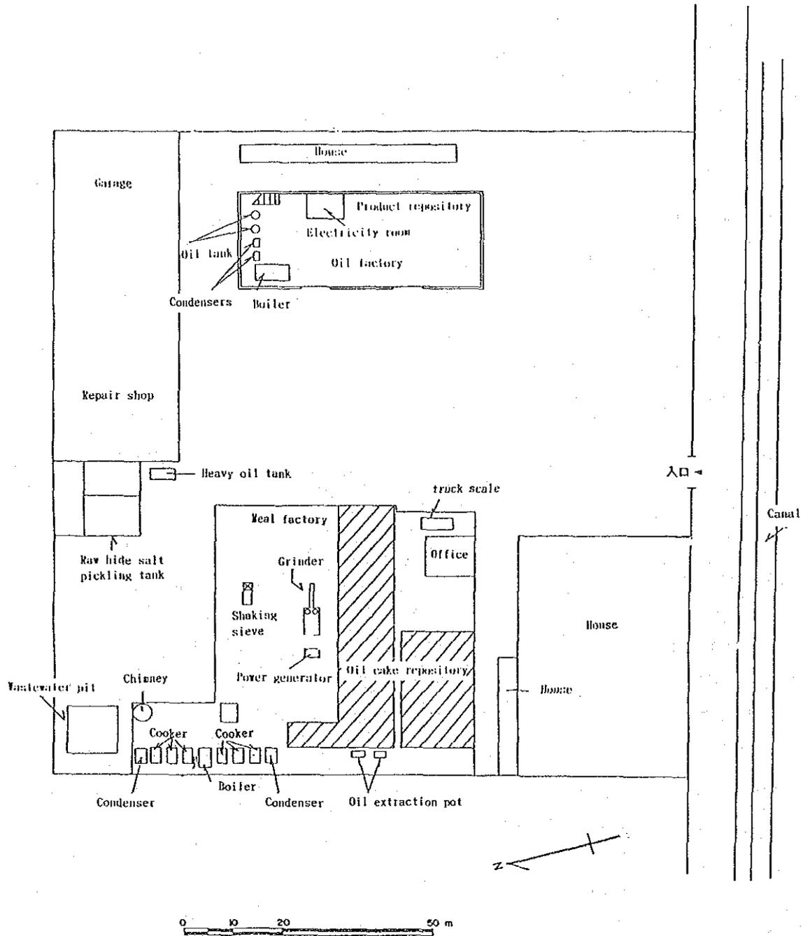
Figure 4-17 Layout of the Factory (Bone Meal Plant C)
