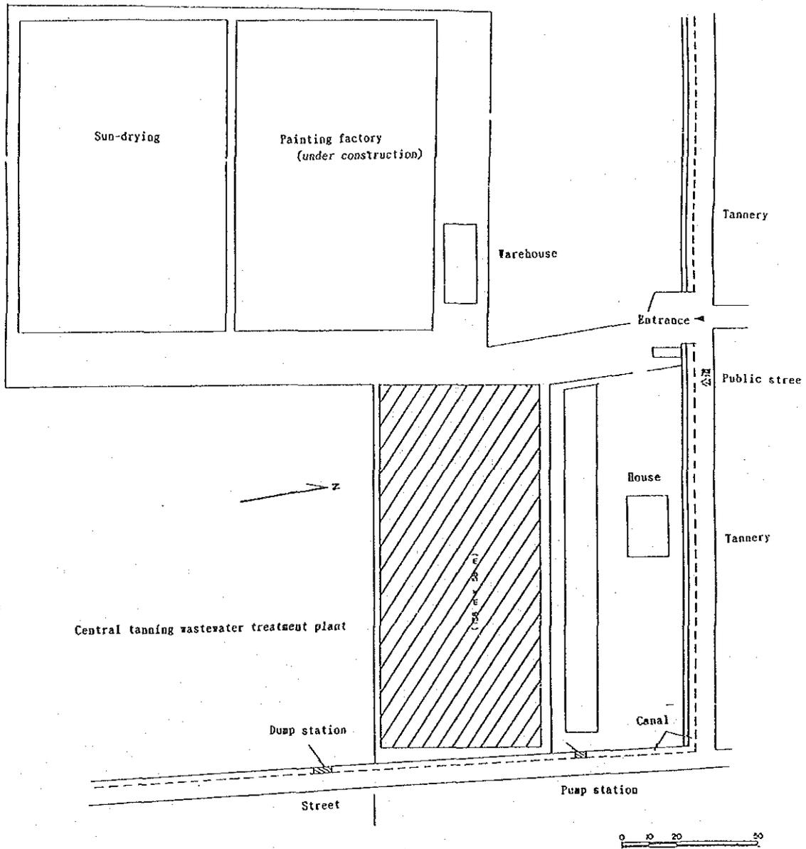
Figure 4-29 Site Plan of the Factory (Tannery F)
