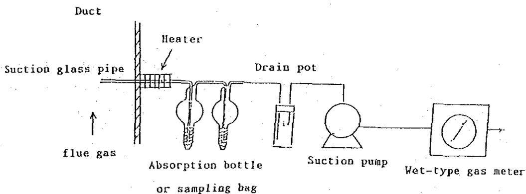
In case of gas sampling in a flue, suction flow rate was also measured by means of a pito-meter, together with measurements of pressure, temperature and water content.
