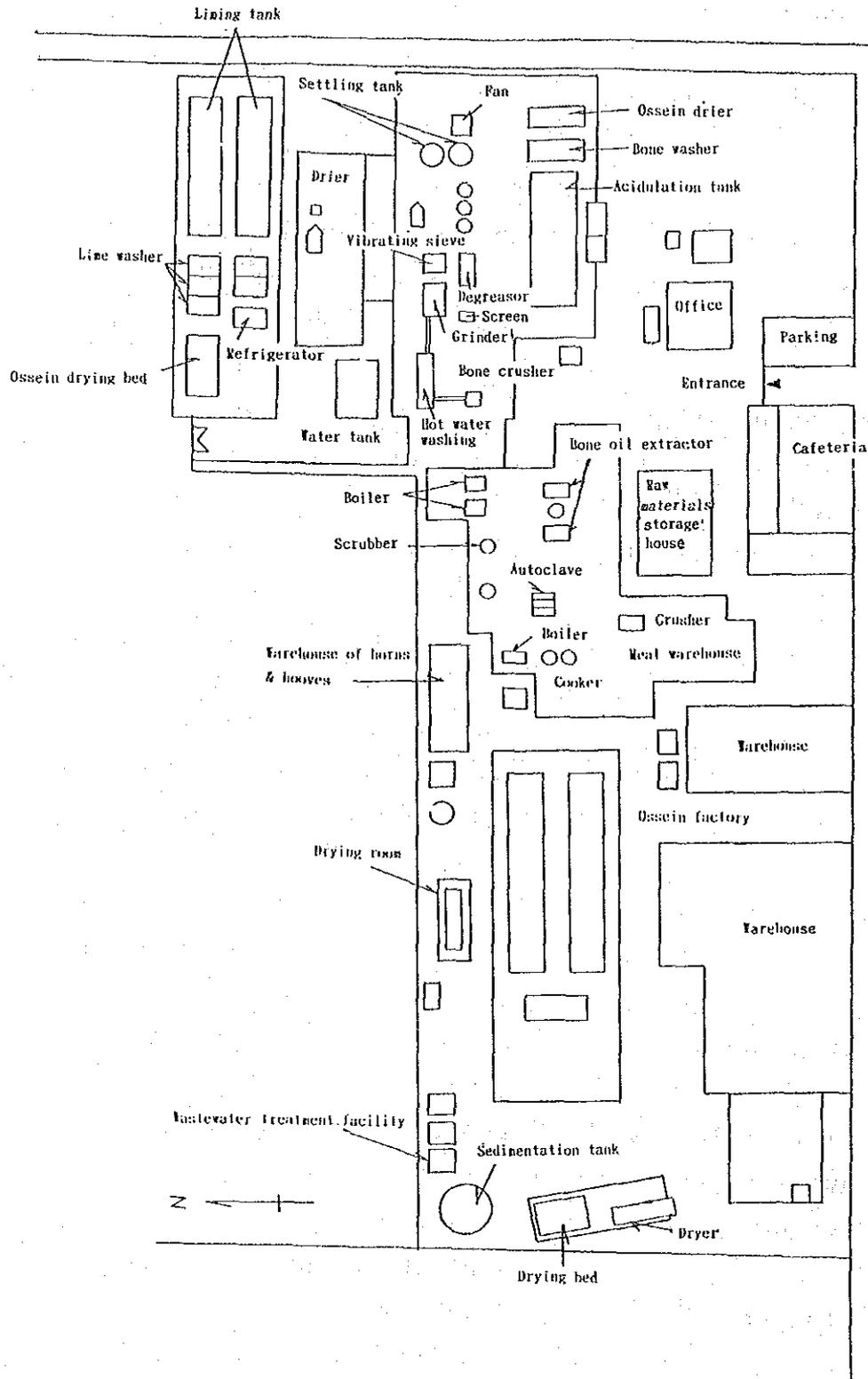
Figure 4-21 Layout of the Factory (Bone Meal Plant D)
