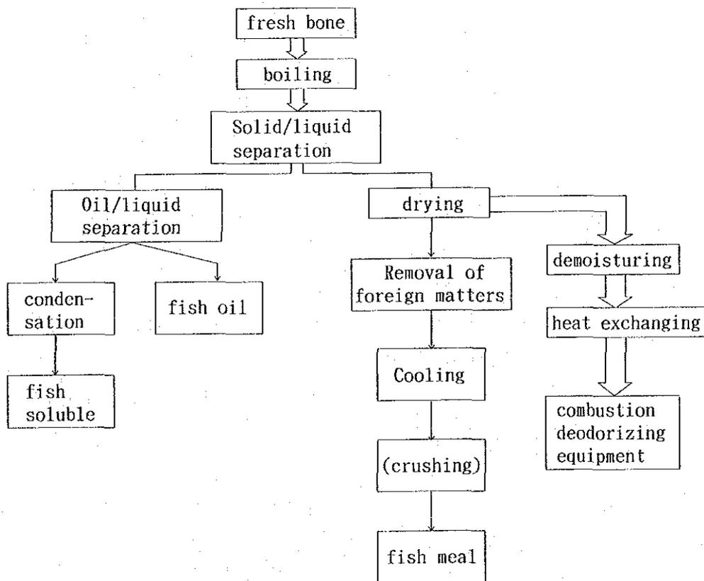
Figure 5-12 Process of Fish Meal Production
