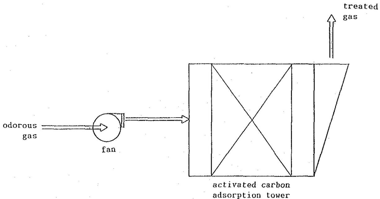
Figure 5-8 Schematic of Activated Carbon Adsorption
