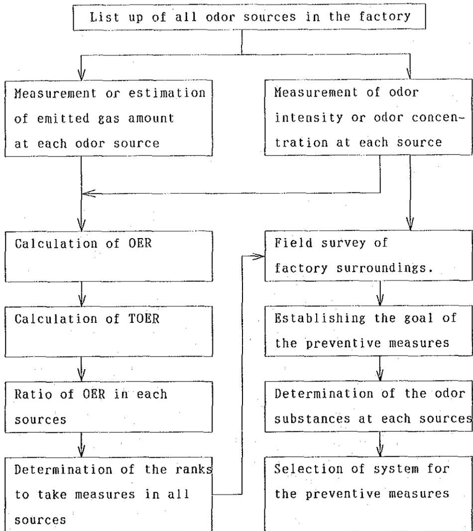
Figure 5-1 Flowchart of the Survey and Planning of Odor Prevention
