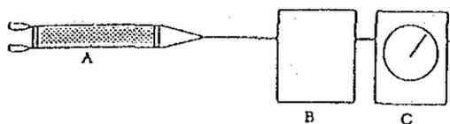
A: Gas sampling tube      B: Suction pump
