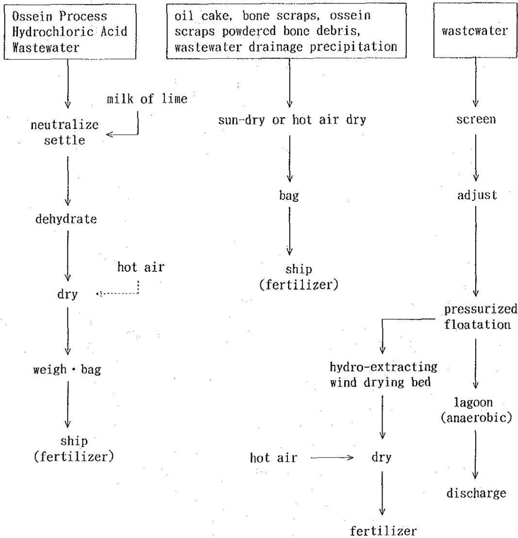
Figure 4-22 (3) Production Process (Bone Meal Plant D)
