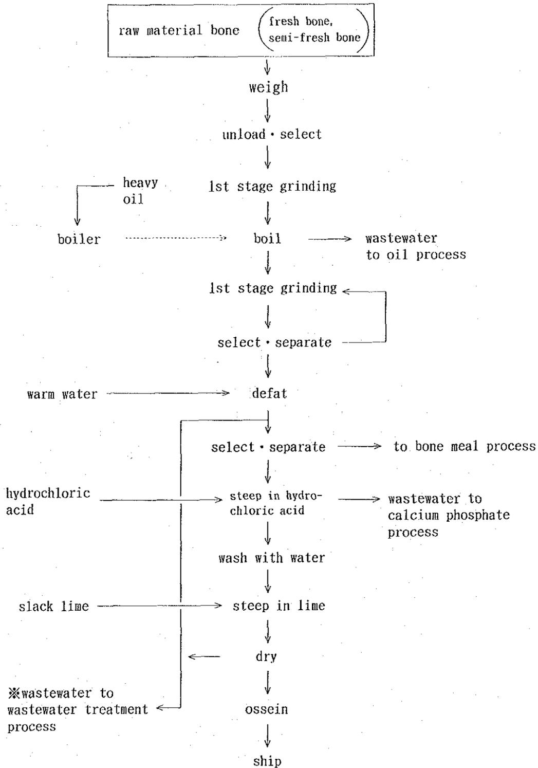
Figure 4-22 (1) Production Process (Bone Meal Plant D)
