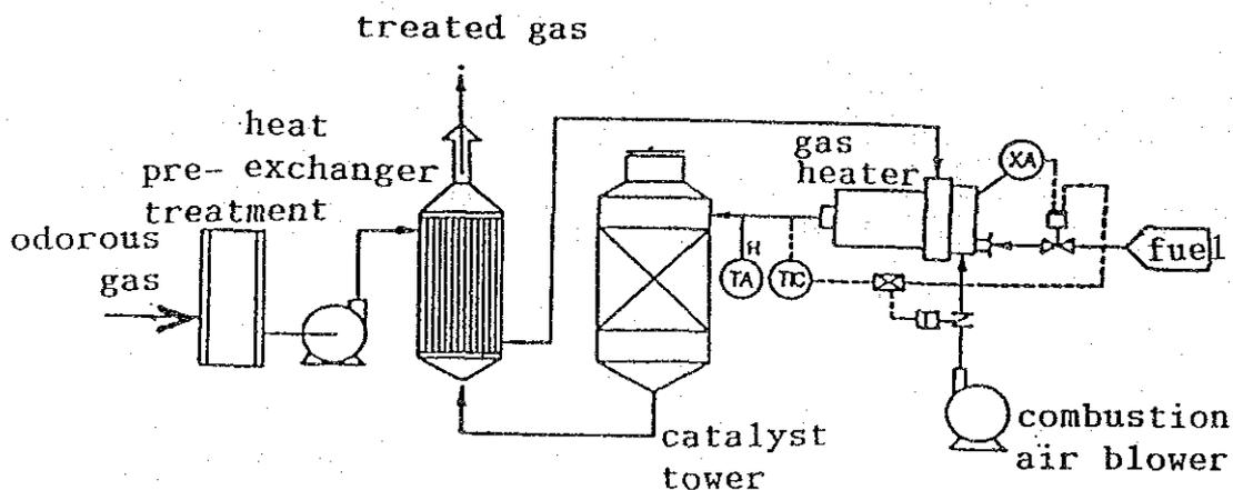
Figure 5-11 Schematic of Catalytic Combustion
