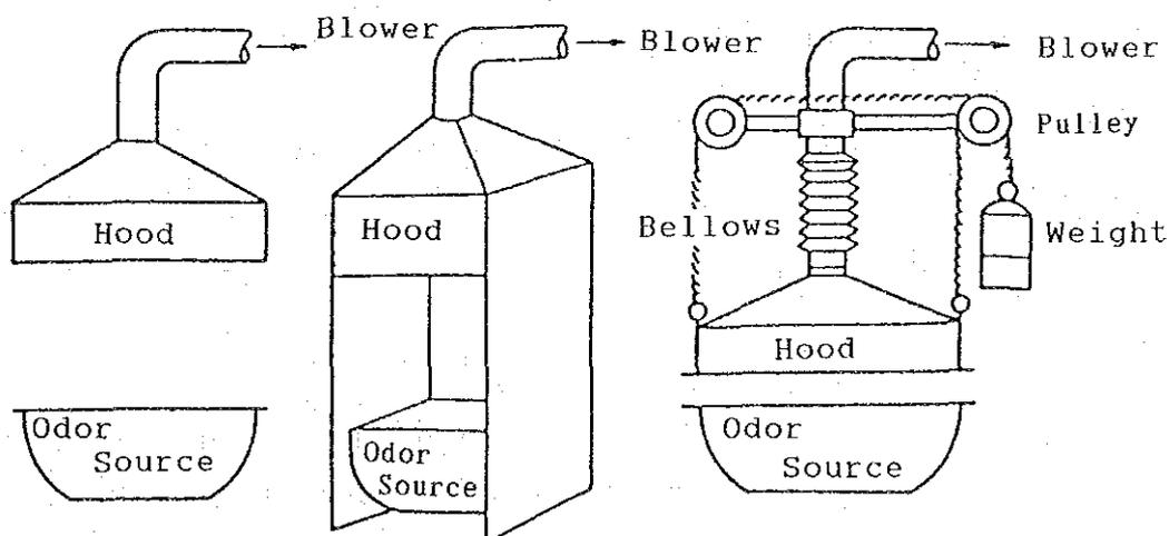
Figure 5-3 Odor Trapping by Use of Hoods at Odor Source
