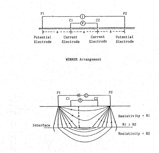
Lines of Current Flow between Electrodes P1 and P2 in Two-Layered earth
