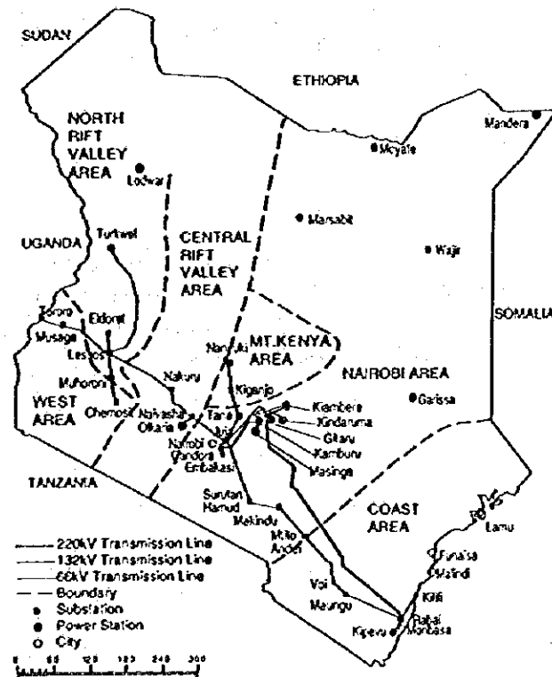
Figure A. 37 National Power Grid
