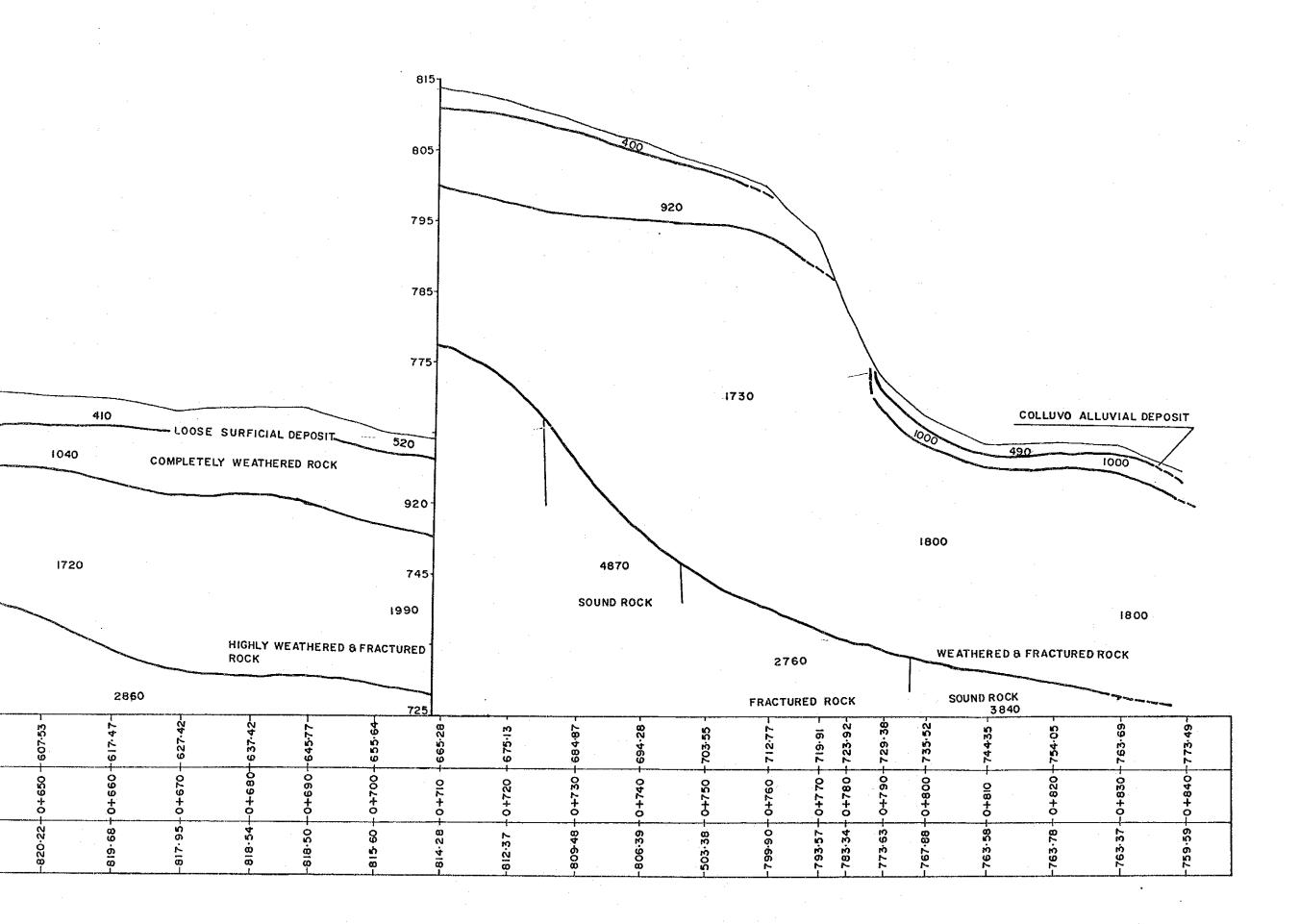
SEISMIC DEPTH SE
