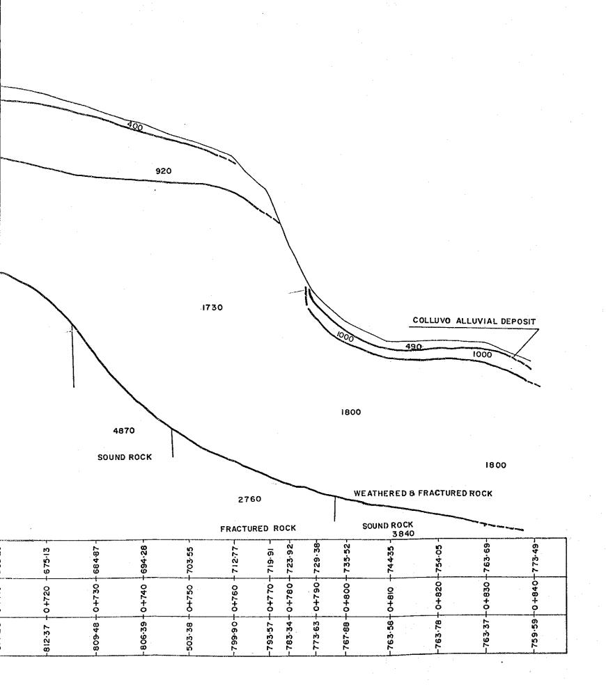
SEISMIC DEPTH SECTION ALONG SL-2
