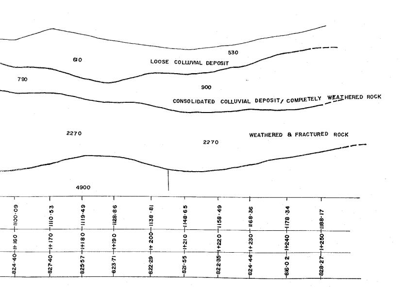
SEISMIC DEPTH SECTION ALONG SL-4
