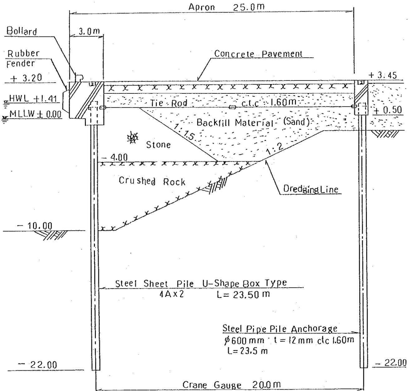
Figure 2-7-4 Typical Cross Section of -10m Container Berth at Batangas Port
