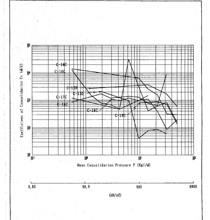
Coefficient of Consolidation, Cv versus Pressure Curves
